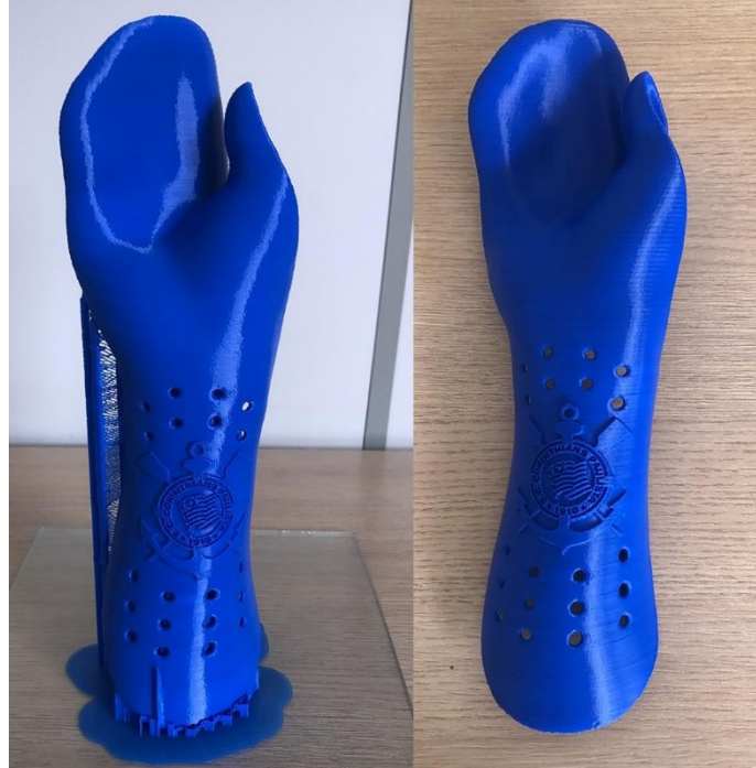
Figure 13. Orthosis with supports (left) and orthosis finished without supports (right).
