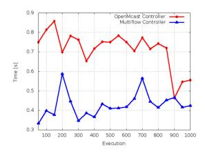
**Figure 4.** Average time from the client join and the receipt of the first packet.
