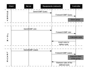
Figure 2. Multiflow operation flow diagram.
